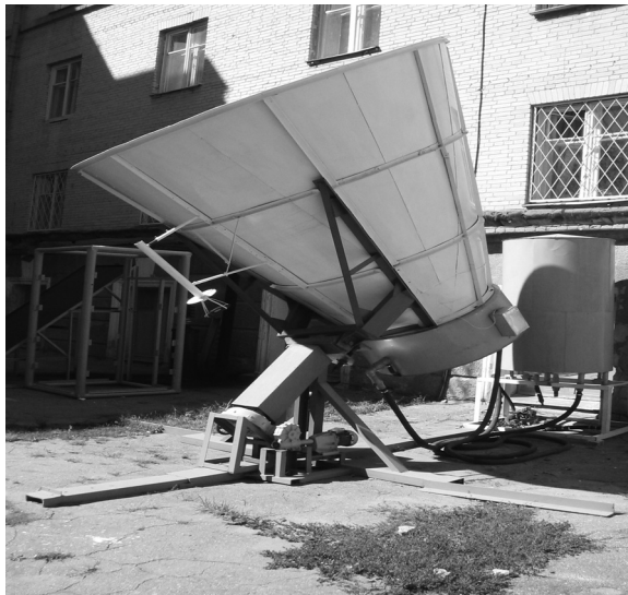
Figure 1. Conical solar concentrator
