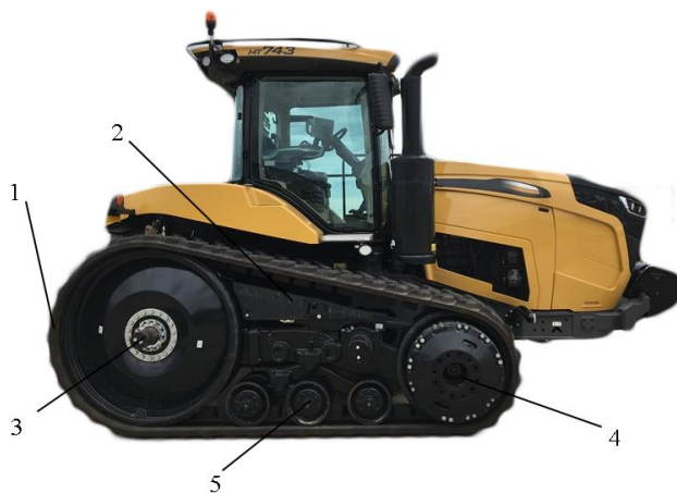
Sl. 35. Traktor Caterpillar sa gumenom gusenicom pozitivne vuče Fig. 35. Caterpillar tractor with rubber track for positive traction
