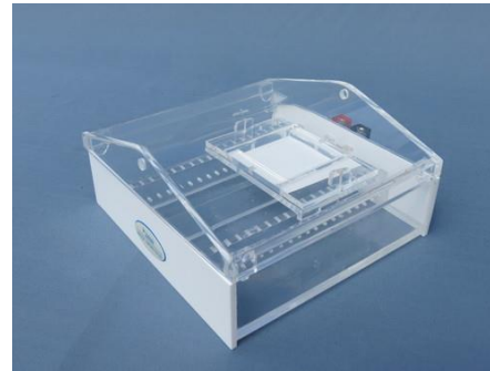
Figure 21 - Apparatus for paper electrophoresis.
