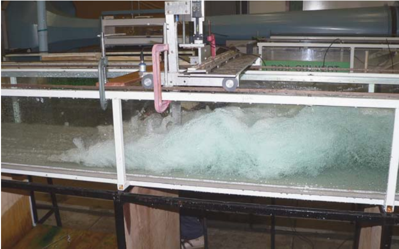
Figure 7.9. Advection of air bubbles in a horizontal hydraulic jump.
