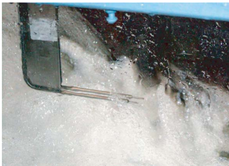
(b) Photograph of two single-tip conductivity probes side-by-side in a hydraulic jump ( Fr_1 = 7.9 , \rho_w \cdot V_1 \cdot d_1 / \mu_w = 9.4 \text{ E} + 4 )—flow from right to left
