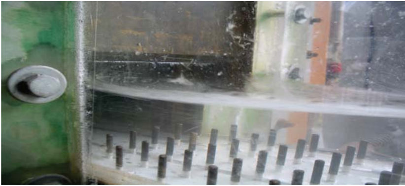
Figure 10.5. View of vegetation obtained through rigid cylinders.
